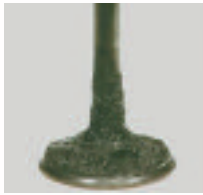
Intake valve before P.i. treatment.
