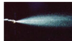
Injector spray pattern after P.i. treatment.
